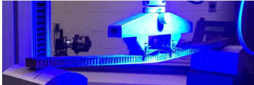
Figure 36: Failure of 8 ply unidirectional delaminated sample
