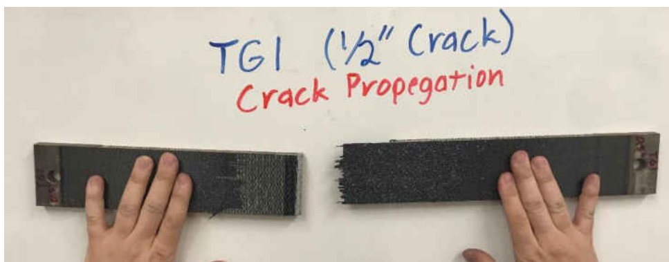
Figure 82: Crack propagation failure of a double lap joint 1/2" defect sample (back)
