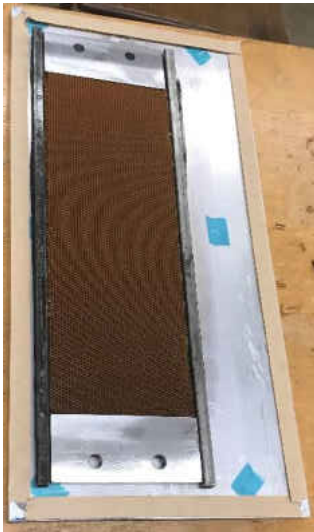
Figure 63: Panel with steel side supports
