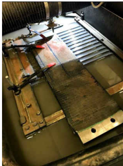
Figure 58: Cutting of double lap joint panel with waterjet machine
