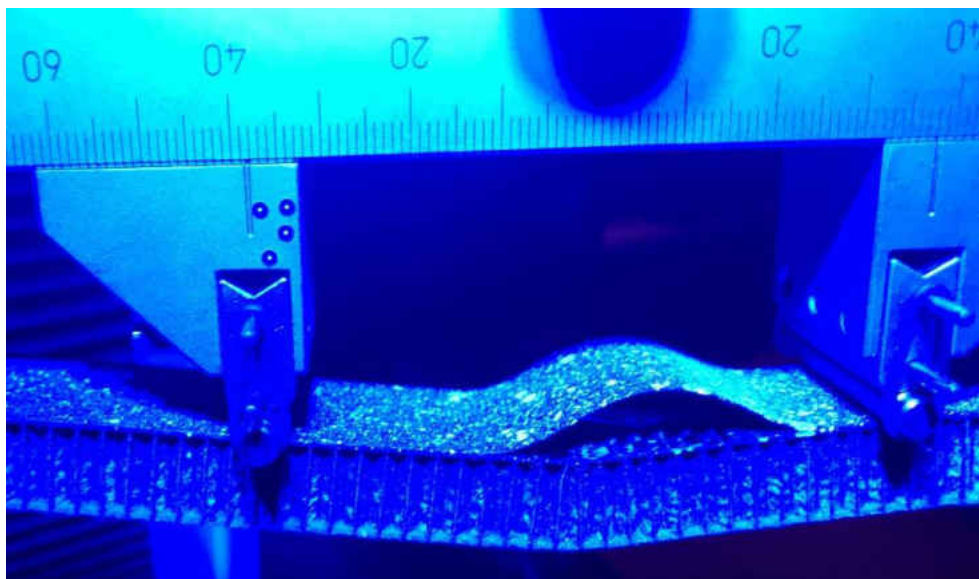
Figure 23: Failure of 4 ply unidirectional delaminated sample
