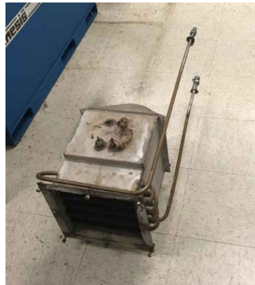
Figure 67: Heating element removed from autoclave
