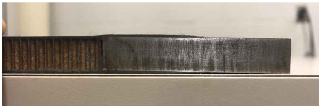
Figure 73: Misalignment of the end adaptor in sample TC2
