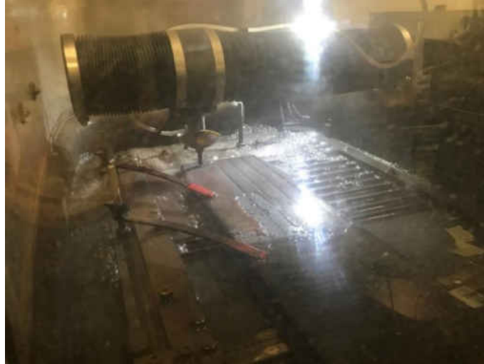
Figure 7: Waterjet cutting of a panel
