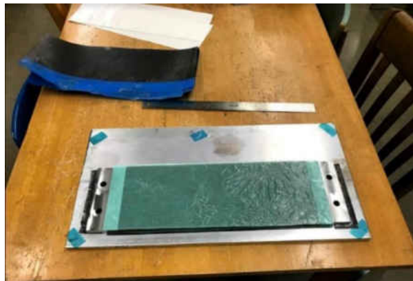
Figure 55: Fabrication of a double lap joint panel
