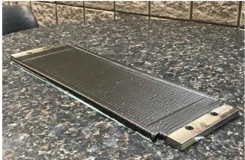
Figure 64: Successful curing of a panel in the autoclave
