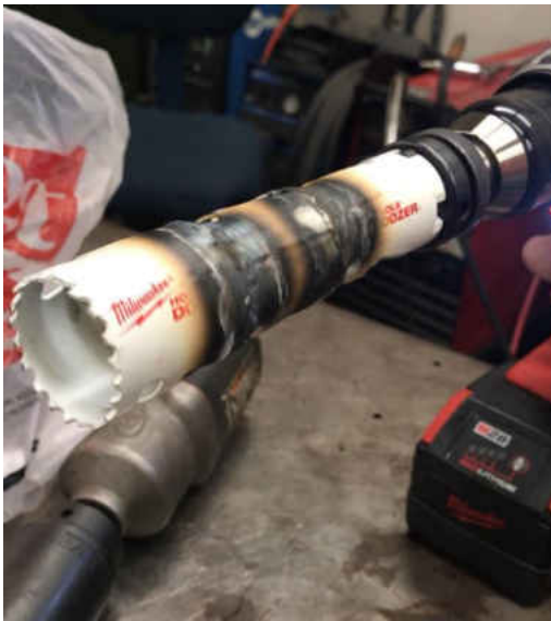
Figure 66: Custom tool made for repairing of autoclave
